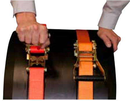
Figure C.24: Tightening of the tension belt
