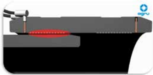
Figure C.18: Principle of the bifilar welding
