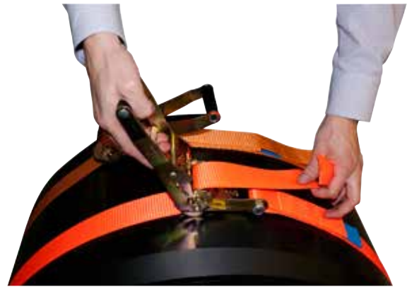
Figure C.25: Opening the tension belt
