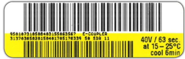
Figure C.12: Agru bar code label
