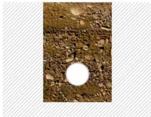
Figure D.3: Diagram of a trench after a sandbed-free installation.
