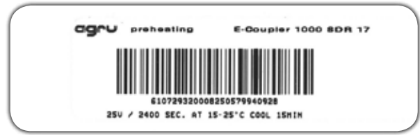
Figure C.19: Agru pre-heating code
