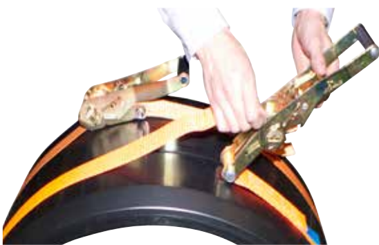
Figure C.23: Mounting the tension belt
