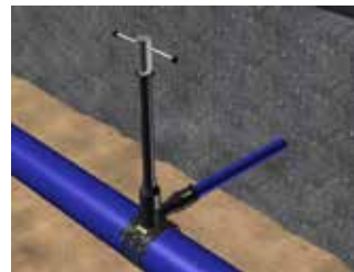
Figure C.41: Tapping of the pipe
