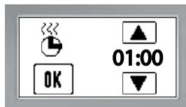
When the session time expires, a high tone buzzer notifies the user. Then the control unit goes to off mode or cabin drying (only with steamer).
