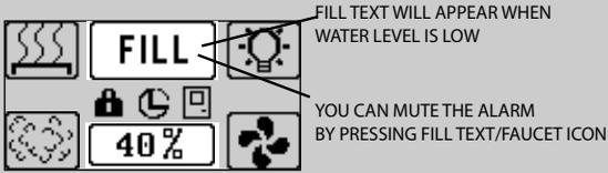
When the water level is low, a low tone interval beep and “Fill” will be displayed to alarm the user.
