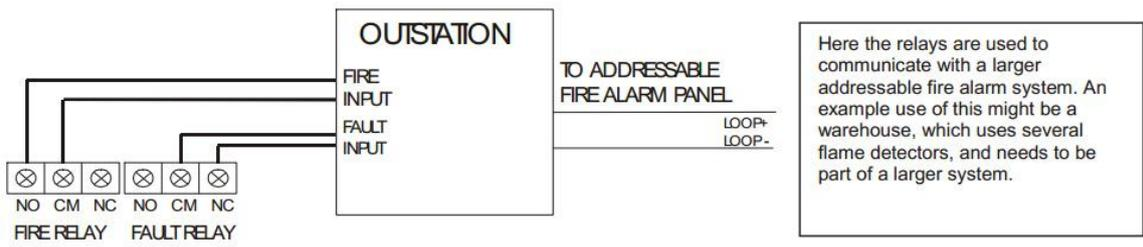
The termination for the above inputs must be as indicated on the main PCB (See page 15). The Earthing of the cable screens should be as shown on page 9.
