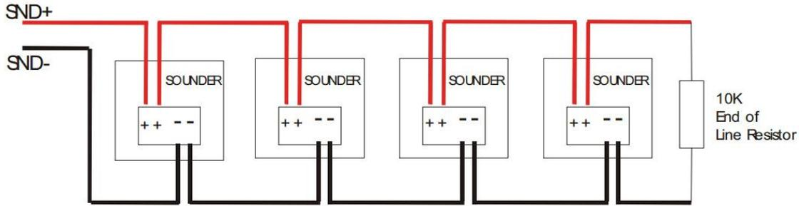
Note: If non-polarised alarm devices (e.g. some types of old mechanical bell, or a relay) are used, then a diode will have to be placed in line with the device to enable fault monitoring. They may also need a back EMF protection diode.
