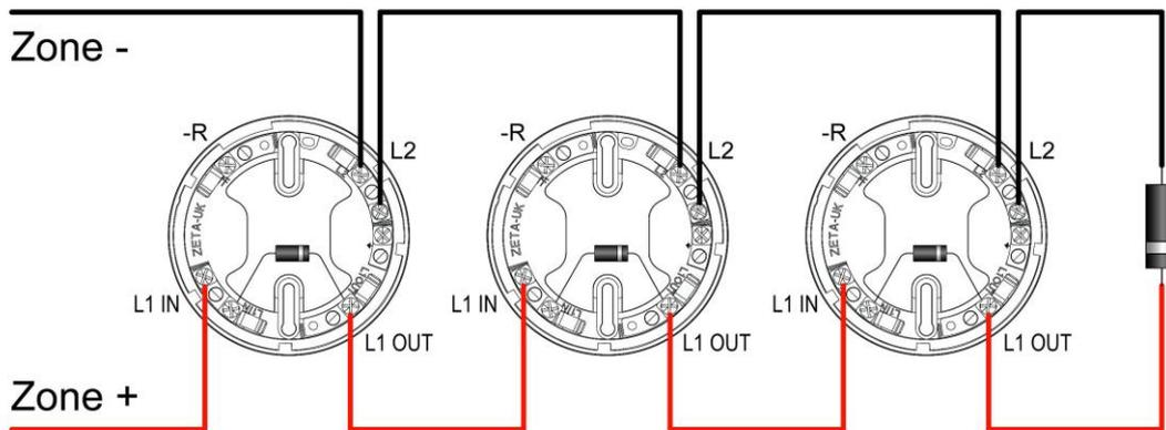
An End of Line diode (provided in the Panel) must be connected across the terminals of the last device on each circuit to allow the wiring to be monitored. It is polarity sensitive, and connected cathode (STRIPE) to +ve
