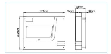
The Infinity 8 control panel is housed in the most attractive, modern designed, flame retardent ABS enclosure, utilising a switch mode power supply. It has a fully removable front cover which improves ease of access for cable installations.
